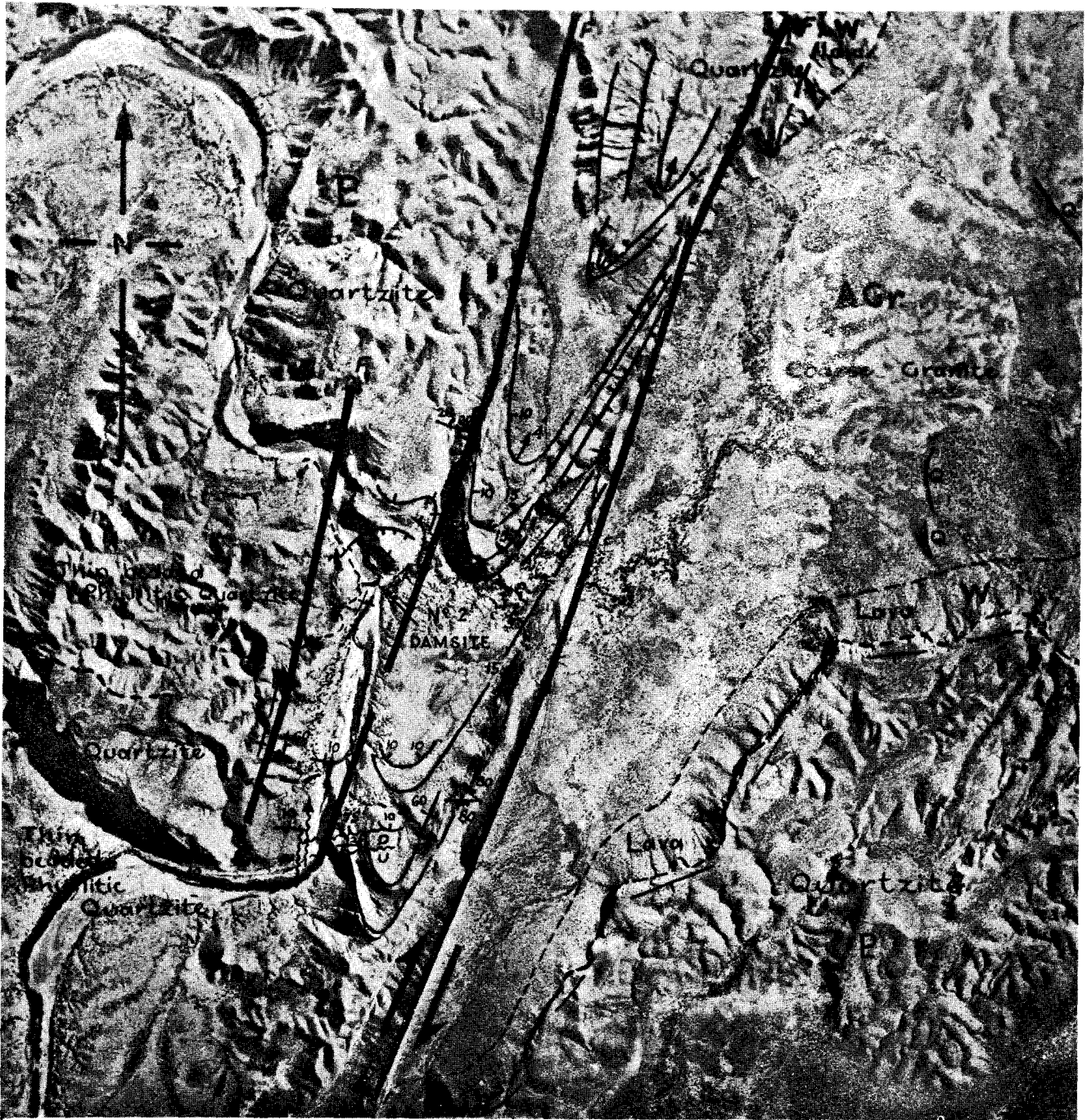
G. S. W. A. DIAGRAMMATIC SKETCH PLAN SHOWING GEOLOGY, REGIONAL FAULTING AND STRUCTURE IN VICINITY OF ORD RIVER MAIN DAMSITE EAST KIMBERLEY Scale : Approx. 60 chains to inch
