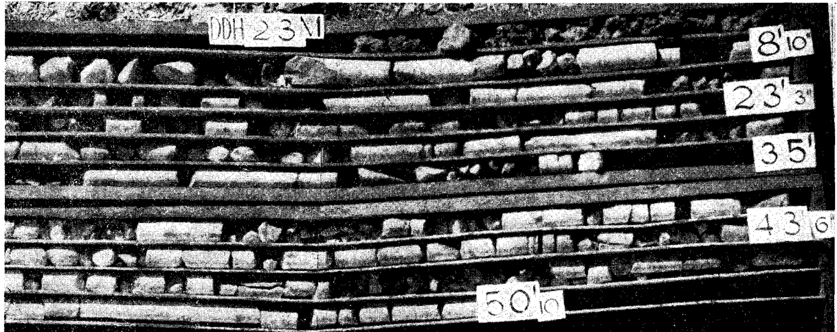
Fig. 6. Core recovery from Bore 23M.
