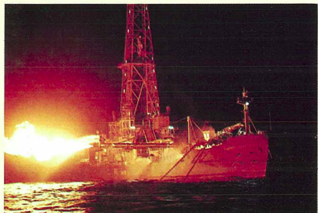
Flaring gas during testing at Wilcox No.1 discovery well in the offshore Carnarvon Basin (Woodside Offshore Petroleum Pty Ltd photo).
