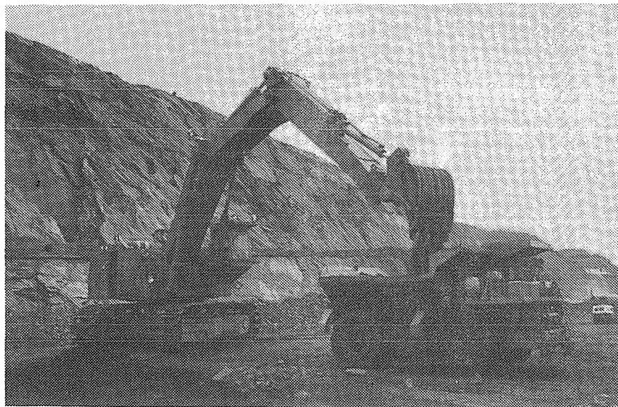
Loading iron ore from the bottom bench (below sea level) at Cockatoo Island — Dampier Mining.
