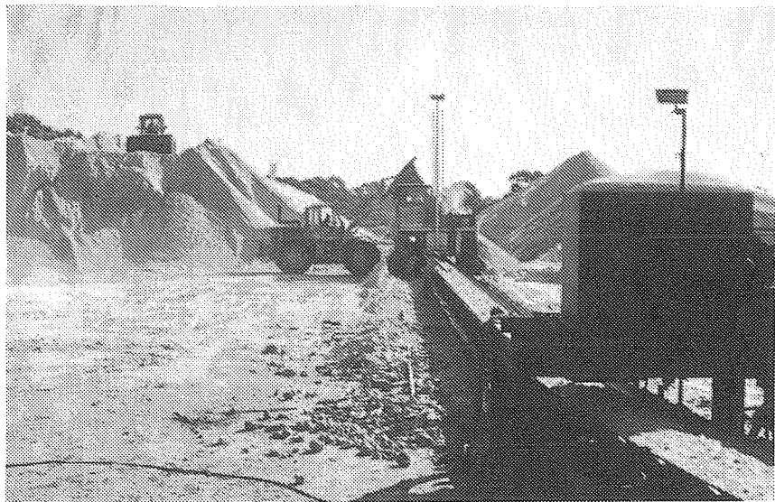
Gypsum from Southern Asiatic Enterprises' Lake Cowan deposit being loaded from port stockpile onto conveyor at Esperance.
