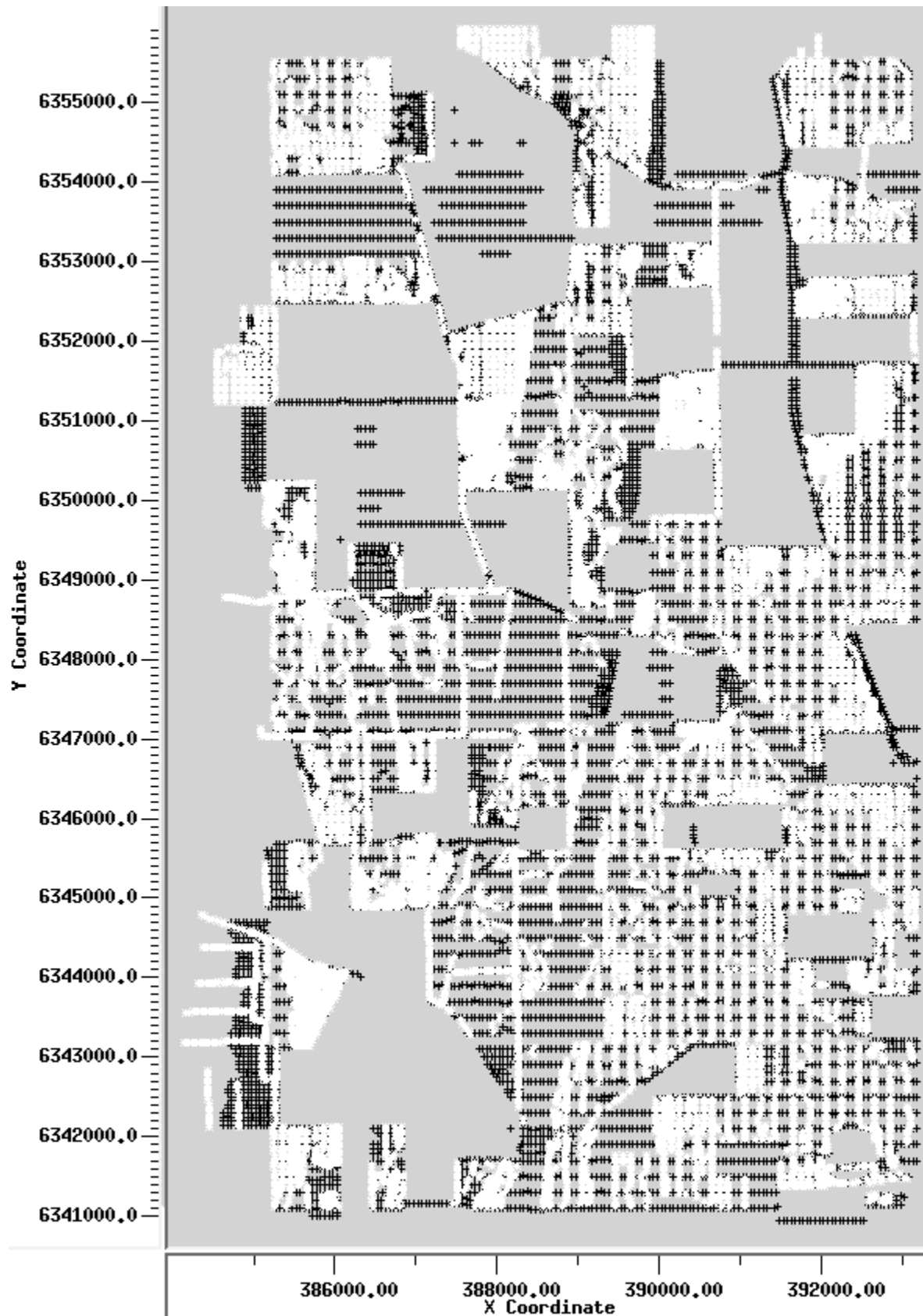
Figure 2. Harvey 3D seismic survey layout for Source (white) and receiver (black) locations where X and Y coordinates are Easting and Northing, respectively. Distances are in metres.
