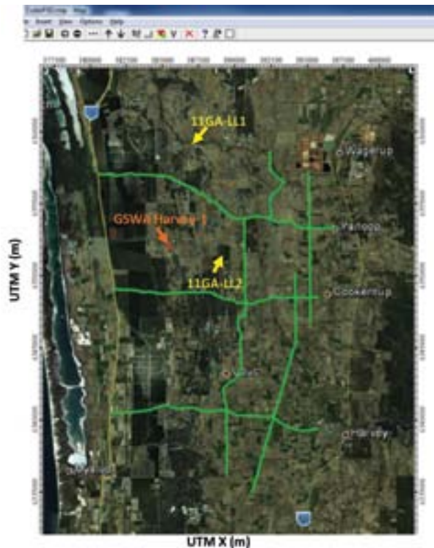
Figure 12 Location of Harvey 1 and the 2D seismic lines run along a series of roads in the region to obtain preliminary information on the structure of the deep subsurface to locate the Harvey 1 well.
