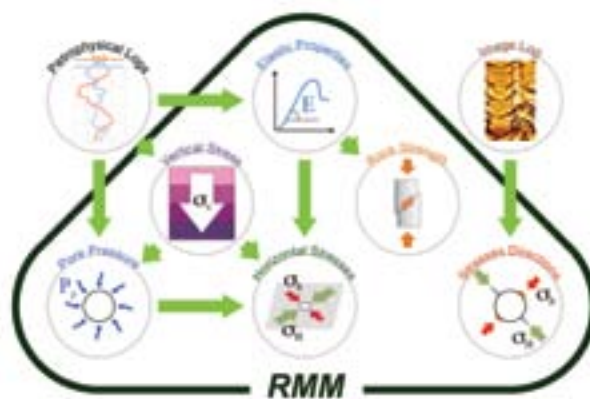
Figure 14 Work flow used to build a Rock Mechanical Model. Figure from Pevzner et al. (2013).
