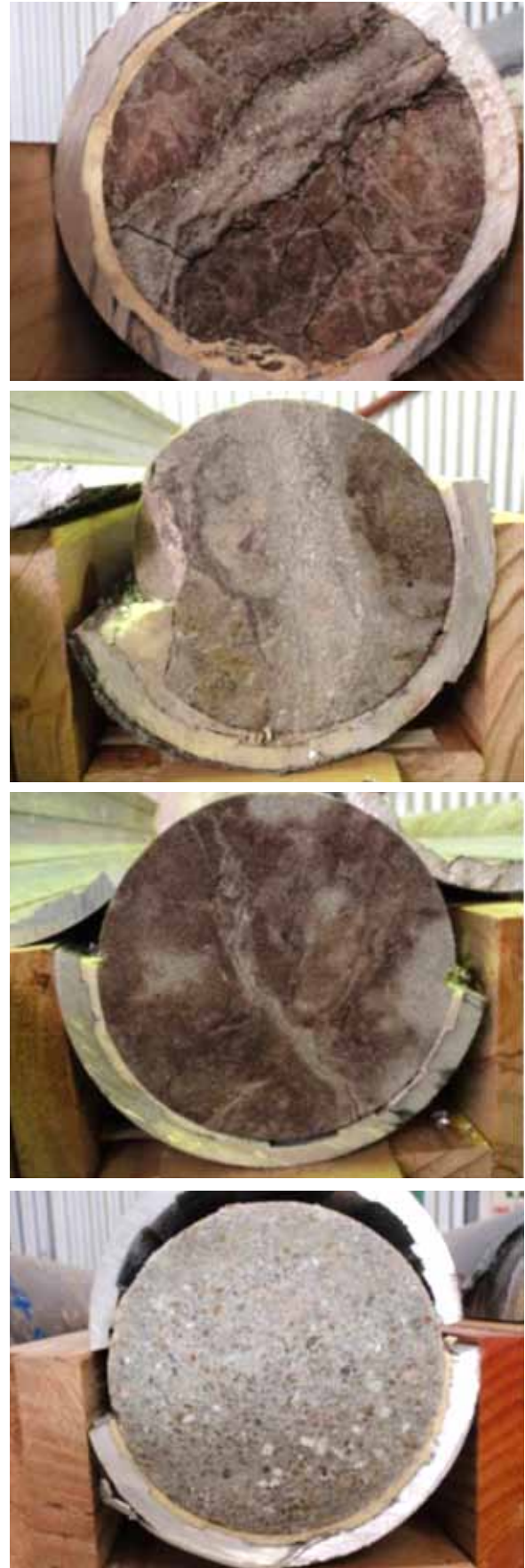
Figure 4. Harvey 1 core samples from the Lesueur Sandstone; from top, Yalgorup Member at 1335m, at 1336m, at 1337m and Wonnerup Member at 2491m.
