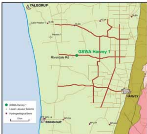
Figure 3. Site map showing the Lower Lesueur 2D Seismic Survey lines, the Harvey 1 well location and water bores along the Harvey and Binningup lines.
