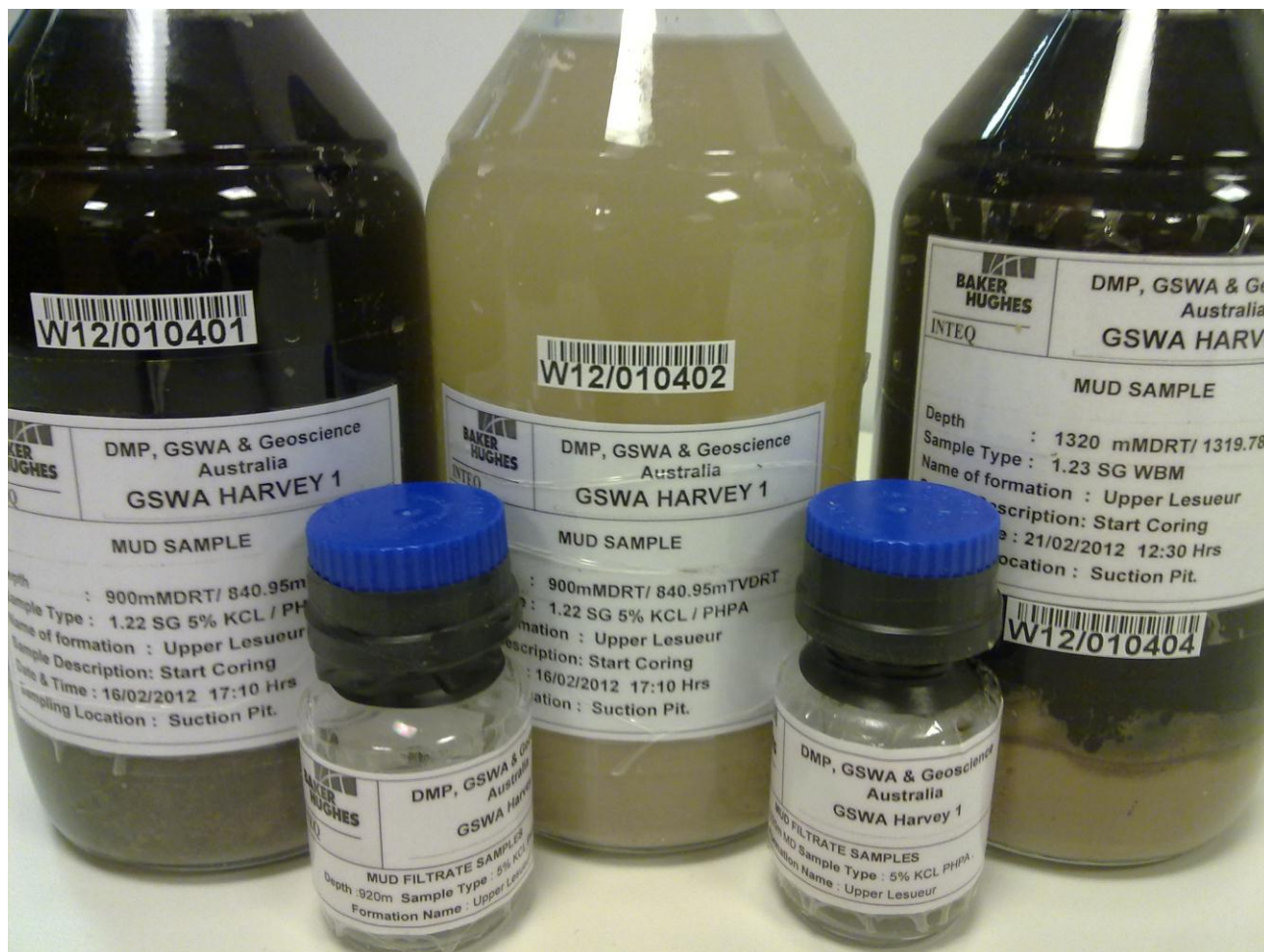
Figure 8 Photograph of the first batch of drilling mud samples received from GSWA. Note the differences between the two 900m mud samples provide at the back left of the photograph.
