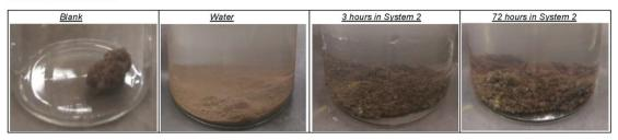
BOX 13 = Brittle, dispersive clay, System 2 provides some encapsulation however nowhere as well as System 1 to stabilise this formation
