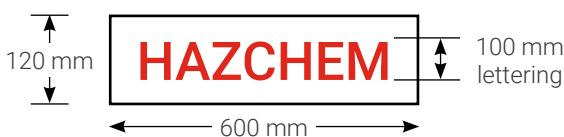
Figure 2 Sample outer warning placard
