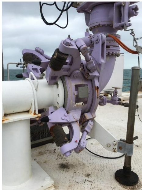
Photograph of the loading arm coupler
