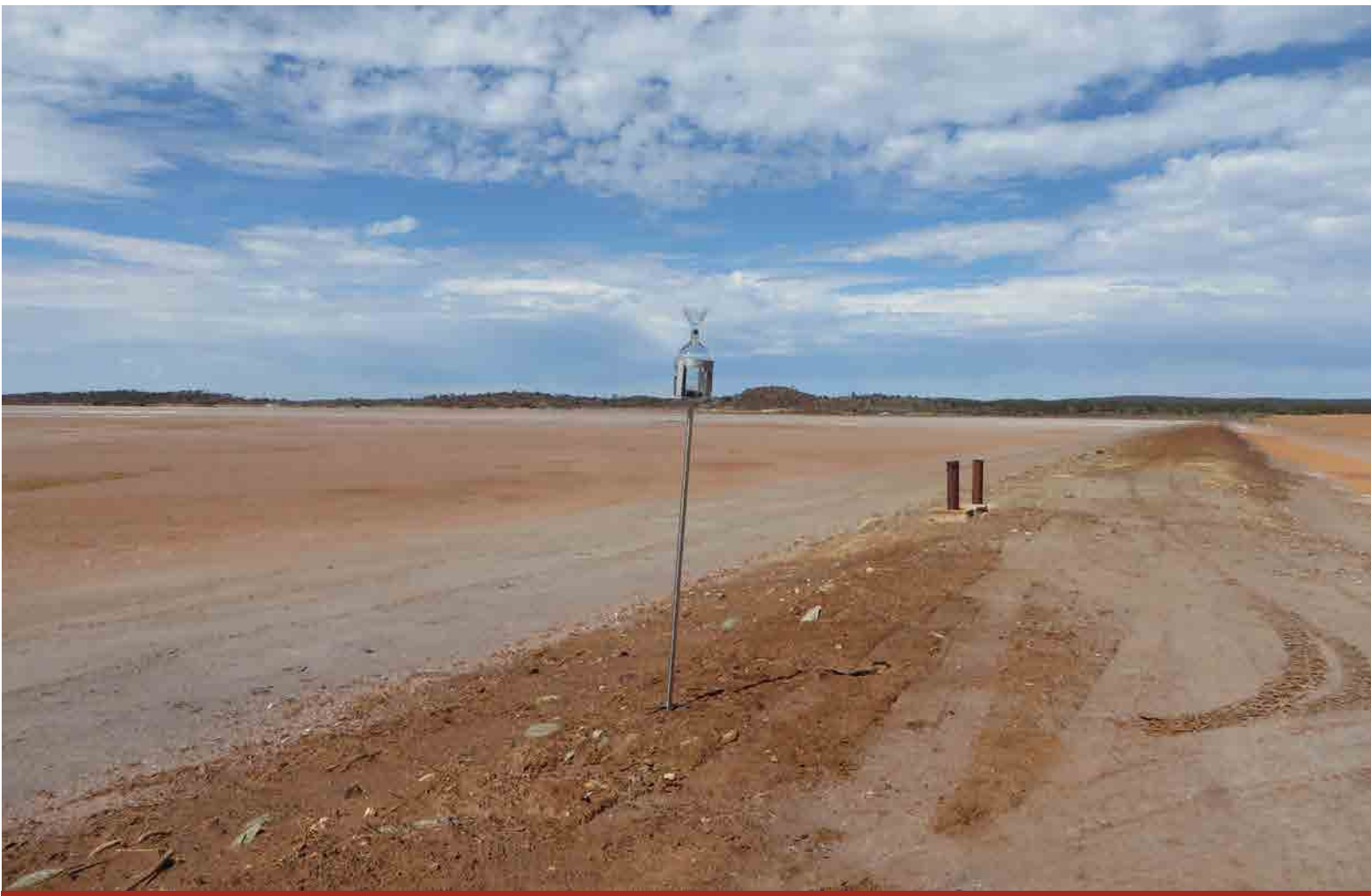
Image 1 - Dust monitoring gauge south of the evaporation pond
