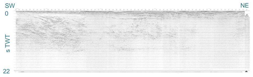
Crustal seismic reflection signature typical for Yilgarn Craton: Upper crust – weakly reflective Middle and lower crust – strongly reflective
