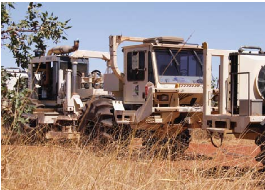
Vibroseis trucks from the Bunda 3D seismic survey in the Canning Basin in 2010 (Photo courtesy of Buru Energy Ltd)
