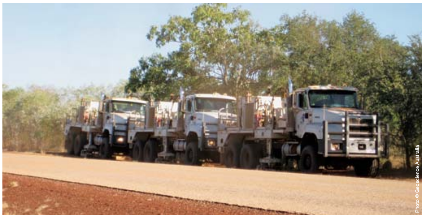
Seismic Energy Source: 3 X Hemi 50,000 pound vibrators
