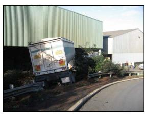
Also, at a mine in Queensland, an unattended partly loaded explosives truck was parked with its engine running. The operator had applied the park brake before disembarking and was walking away from the truck when he noticed it moving. While the truck was rolling away he climbed back into the cab and stopped the truck by applying the foot brake. The truck had travelled about 20 metres and ended up with the front wheels suspended over a 2.5 metre drop off.
