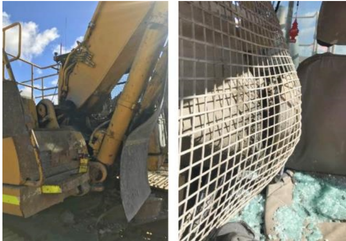
L. Inboard boom ear failure. R. Damaged rock mesh and broken window.
