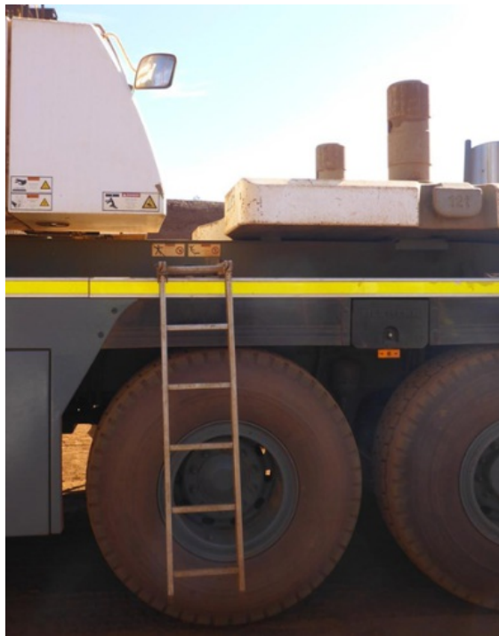
The ladder used to access the crane deck
