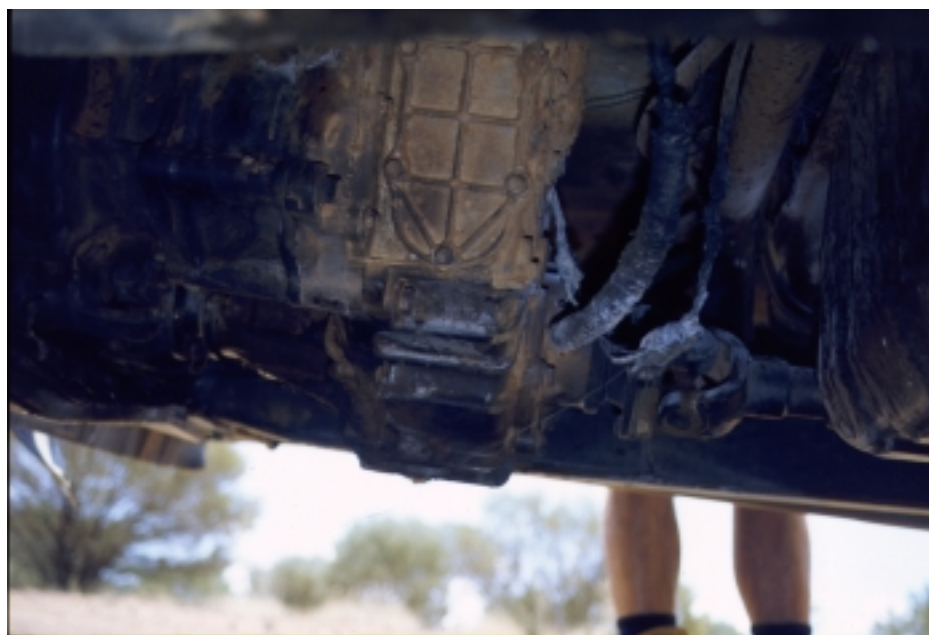
Fire damage to gearbox area shown with guard removed
