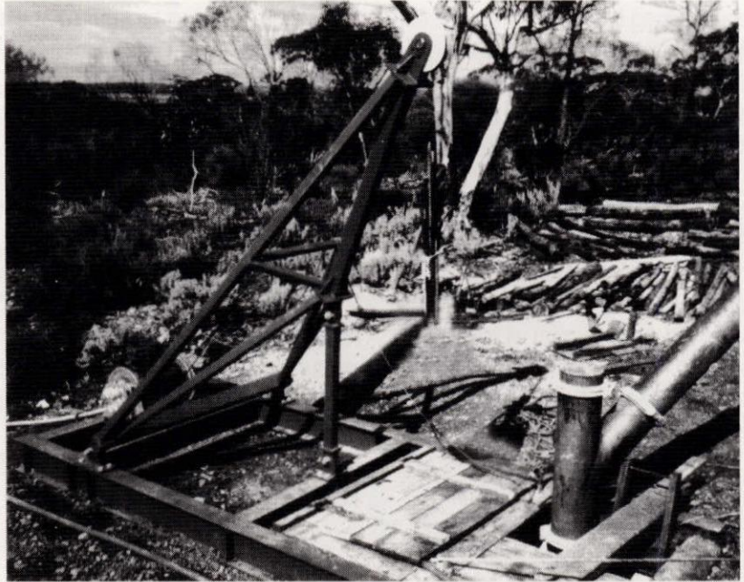
A modern steel 'Whip Pole' used to access an abandoned mine shaft in the Western Australian goldfields.
