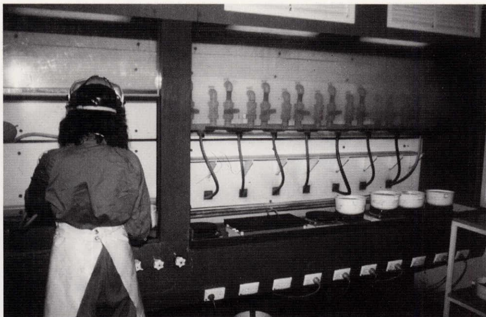
It is mandatory to use HF in a good fume cupboard. This operator who was handling HF had good personal protection equipment, including gloves, faceshield and acid resistant apron in case of spills.
