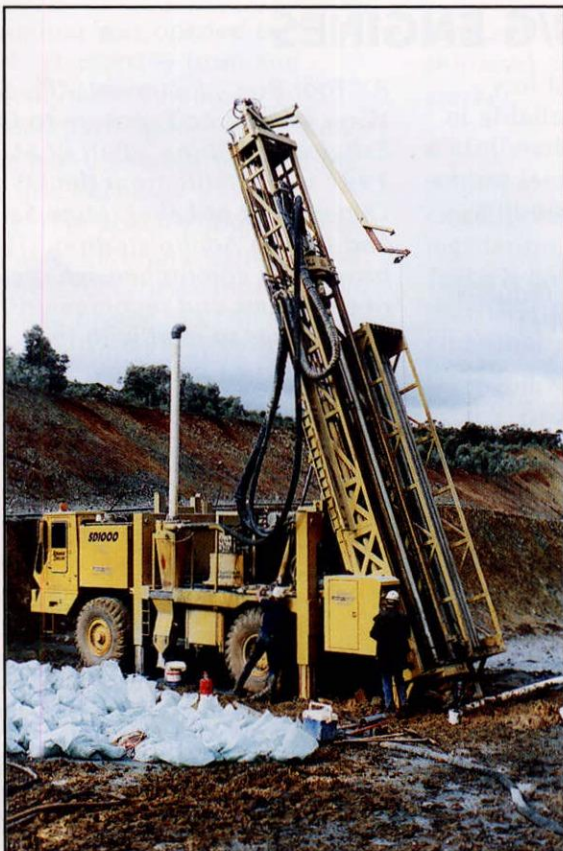
Rear of rig with the rod handling system in use.
