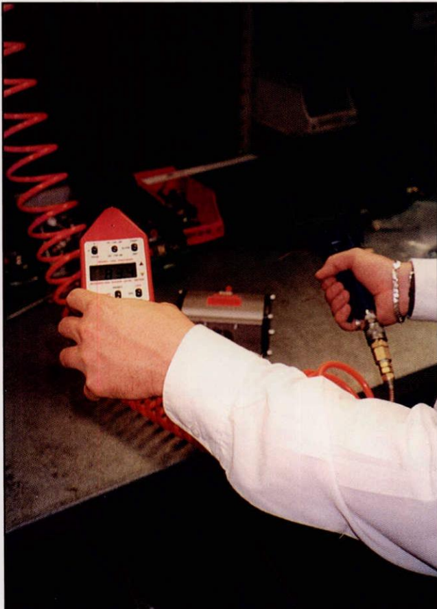
Test on a new blow gun – “A noise level of 83 dB (A) was recorded at the operator’s ear level during normal operations.”
