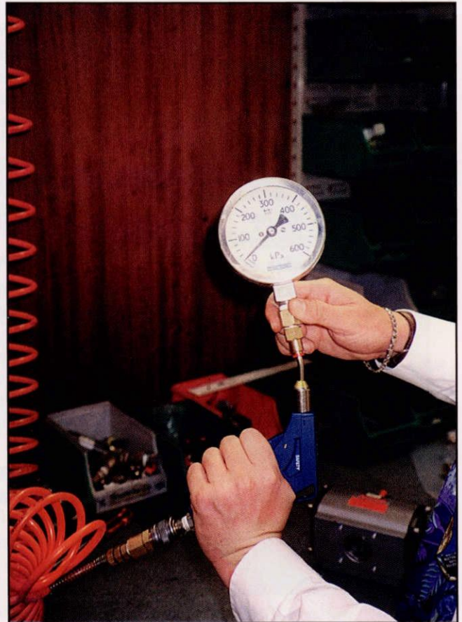
Test on a new blow gun – “When in close proximity to any object, the gun pressure falls rapidly to below 50 kPa.”
