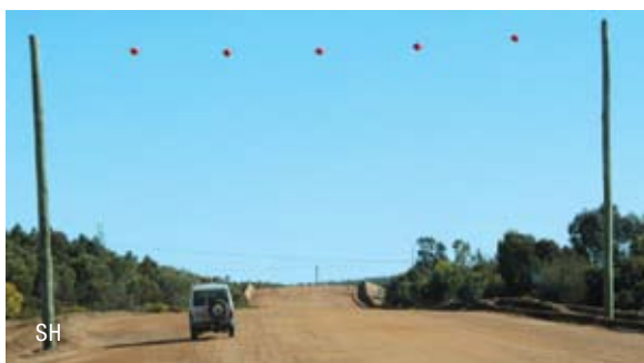
Figure 2 Examples of warning signage (top) and clearance indicator (bottom) on approach to high-voltage overhead powerlines on a mining operation
