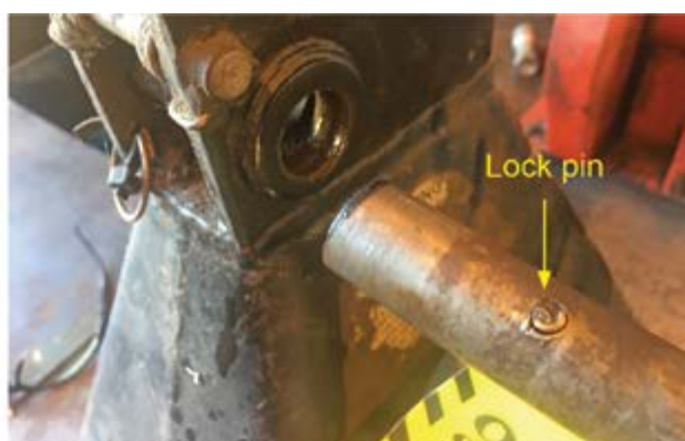
Left. Configuration of a ratchet vehicle support stand. Right. Sheared lock pin located in the locking handle.
