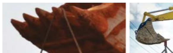
A bucket tooth loaded with a wire rope sling (left) and a soft sling (right).
