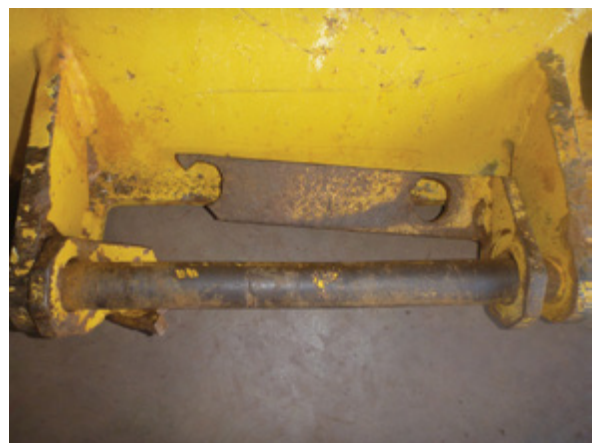
Damaged hinge on left-hand side of belly plate shown after cleaning
