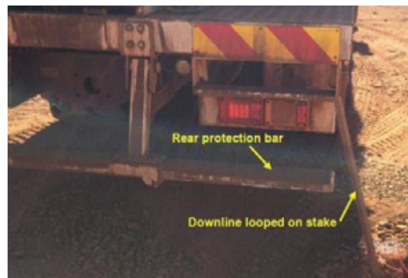
Photograph showing proximity of downline lead and stake to MPU's rear protection bar during loading
