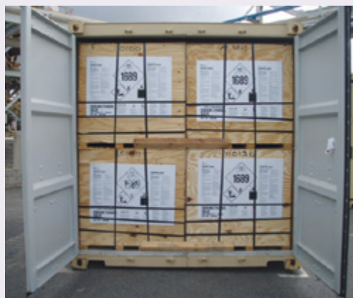
CIBCs of sodium cyanide briquettes in freight container
