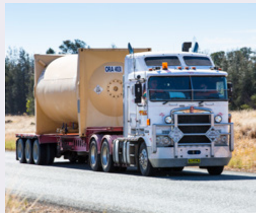
Road vehicle with sparge tank for solid sodium cyanide
