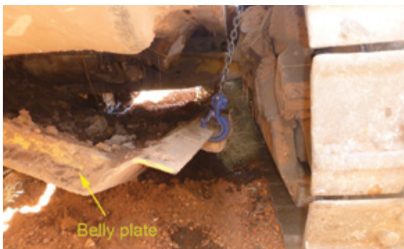
Damaged hinge on left-hand side of belly plate shown after cleaning
