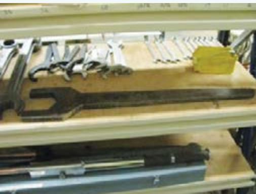
▲ Homemade spanner – how much torque can be applied before it breaks?
