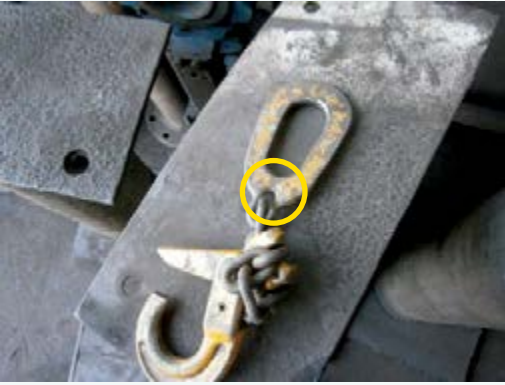
▲ An improvised lifting hook with non-OEM welding – how do you know it will hold?
