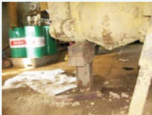
▲ Improvised wooden prop – would you trust it to hold?
