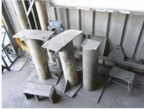
▲ Improvised stands – how stable are they and what is their safe working load (SWL)?
