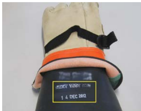
Insulating glove with "next test due" date stamp that was out-of-date as at 15 December 2012
