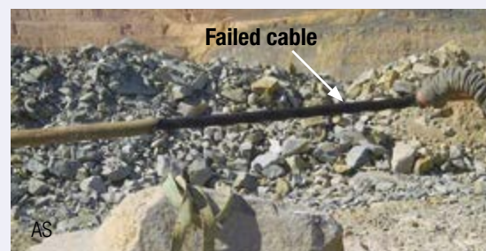
Figure 2b Cable failure due to excessive tension
