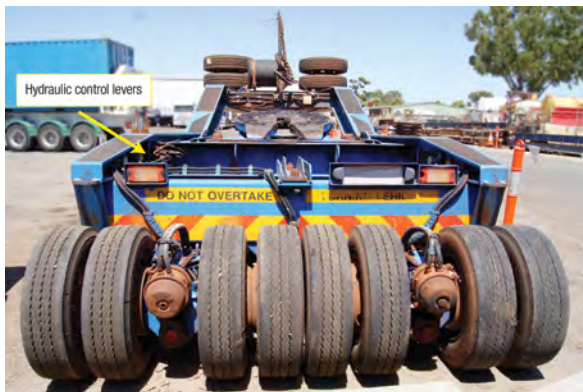
Example of a low loader dolly – note the position of the controls
