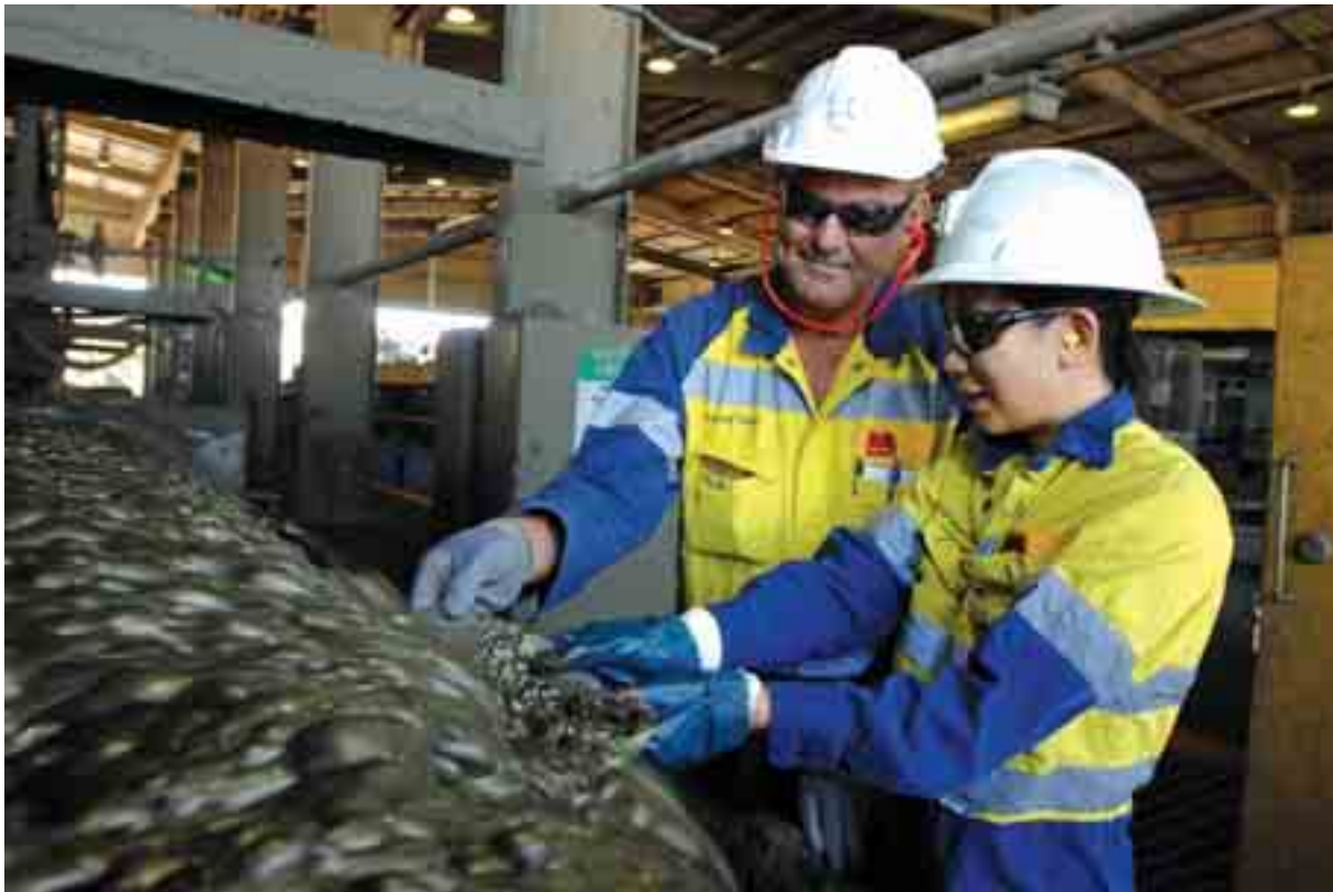
MMG Golden Grove employees take a concentrate sample from the plant flotation circuit.
