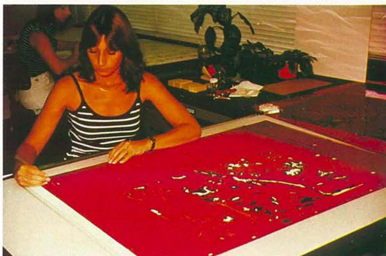
Colour separation using peelcoat
