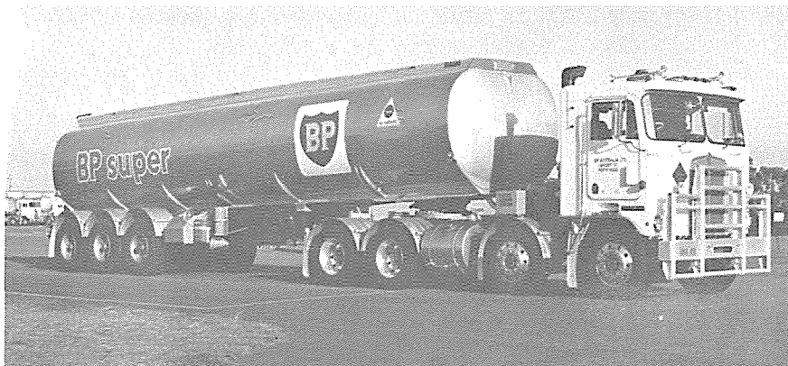
BP Super Tanker (42 kilolitre tanker designed to AS2016:1982).
