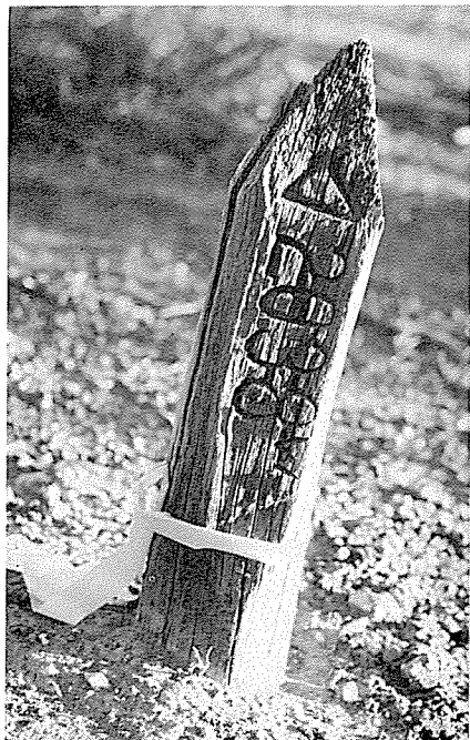
Mulga survey post placed in November 1935 to mark the SW corner of GML 2038W—Ora Banda. Photo: June 1973.
