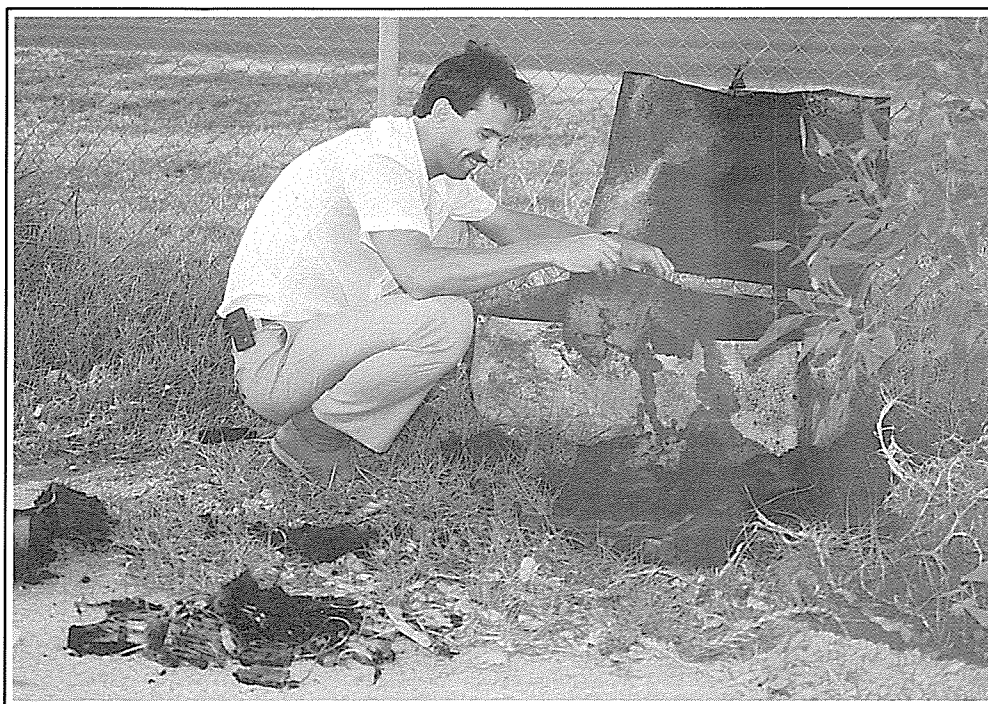
Inspector H. Zuidersma sifts through the burnt out receptacle containing detonators after a fire at a factory in Pinjarra. The owner of the explosives has been prosecuted for the illegal storage of explosives at the site.
