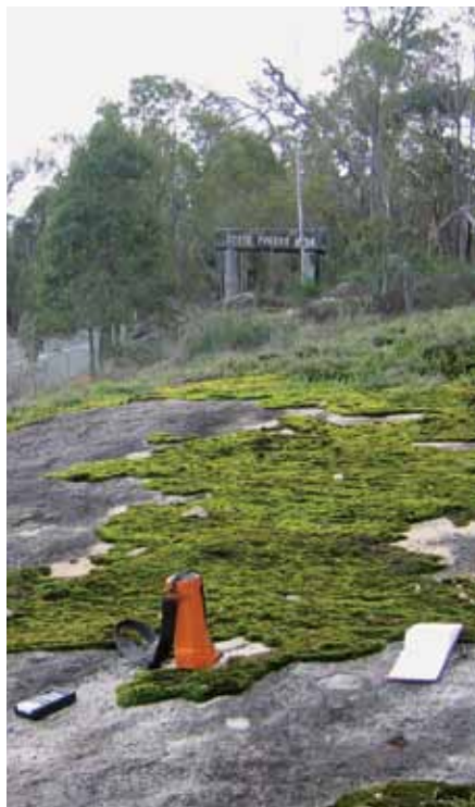
The RS 125 spectrometer (orange) and Geiger counter (black meter) on a roadside granite outcrop near Kalamunda. This site yielded a mean heat generation value of 10.18 \mu\text{Wm}^{-3} , which is one of the highest values observed in the Darling Range
