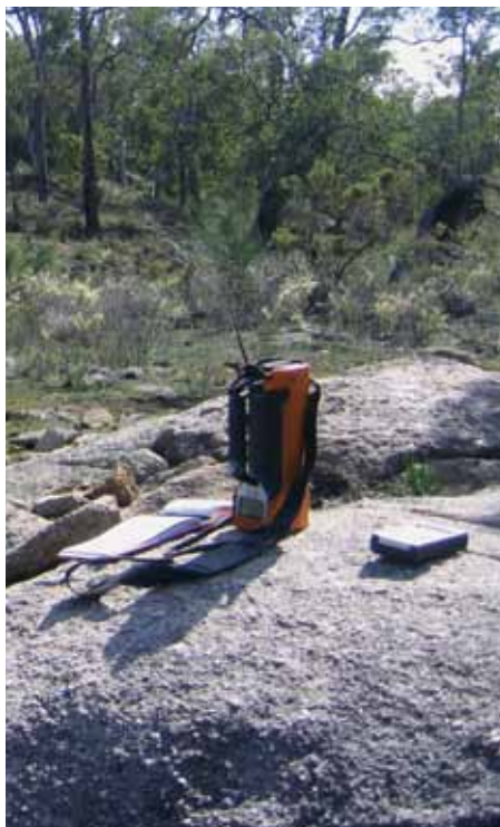
The RS 125 spectrometer (orange) and Geiger counter (black meter) on a granite outcrop near Glen Forrest. Measurements were taken on granite outcrops from fresh to various stages of weathering, and generally very little variation in the radioactive elements was observed with respect to weathering
