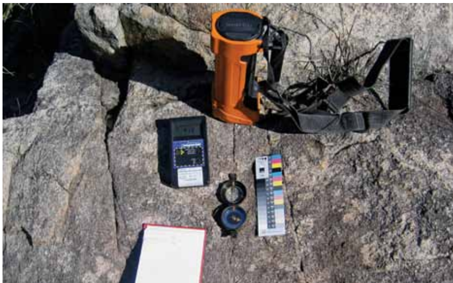
Close up of the recording instruments. The RS 125 spectrometer (orange) with detecting head, containing the detecting crystal, placed on the rock surface, and beside this is a total count Geiger counter (black meter). A compass (to detect fracture orientation), scale and recording book are also shown (Photos courtesy of Mike Middleton)
