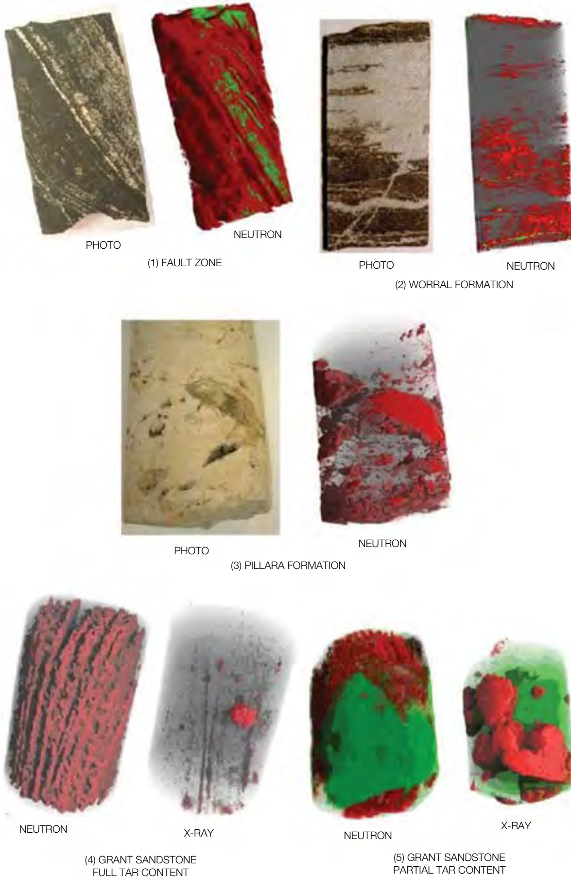
Figure 6 Rocks from the Canning Basin with neutron and X-ray radiographs showing internal structure, where red in the neutron image indicates hydrocarbon (kerogen or residual oil) and red in the X-ray image indicates denser than normal mineralogy
