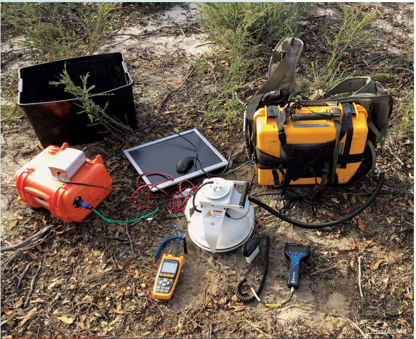
Soil methane flux measuring equipment used by the CSIRO
