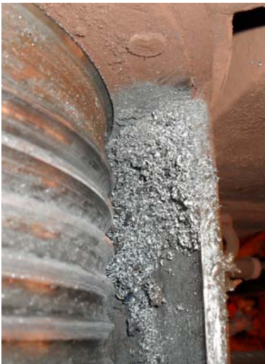
Figure 5 Rope guide shavings
