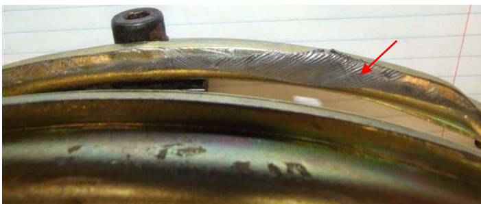
Figure 6 Wire rope imprint
