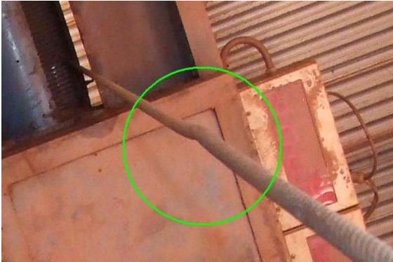
Figure 4 Kink in wire rope
