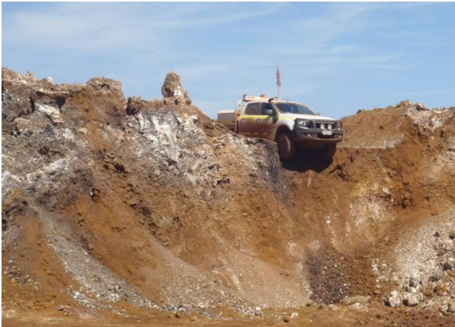
Light vehicle with front wheels hanging over open edge of excavated area
