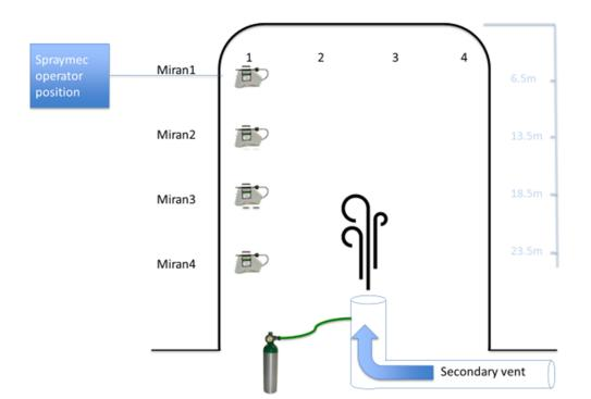
At the **portals** where the experiment was undertaken, it showed no material significant contamination of the intake portal by the exhaust portal. However, there are other portals at Sunrise Dam where the intake and exhaust are closer and thus it would be worthwhile repeating the portal interaction experiment for these sections of the mine to identify if there is any material contamination of the intake
