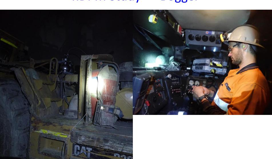
The tracer gas study of a number of underground mining activities, such as charging, bogging, hydro-scaling, shotcreting and truck driving, demonstrated that during those activities there were consistently higher SF6 concentrations measured during the hydroscaling and shotcreting activities.
