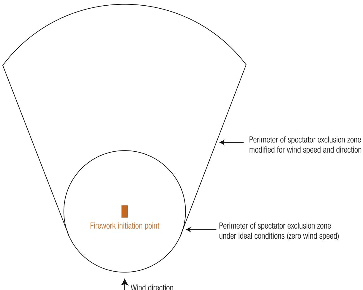
Figure 6.1 Example showing effect of wind on the spectator exclusion zone
