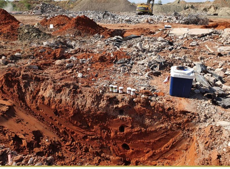
Sampling the soil profile underneath what was the E9 fuel farm to determine the presence of hydrocarbons.
