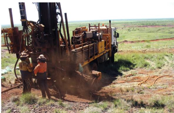
RC wet drilling (water injection)
