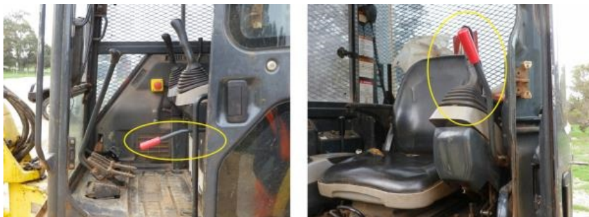
Example of a hydraulic lock-out lever. Left: Unlocked, controls operational. Right: Locked, controls non-operational (Note: Lever position and operation may differ depending on manufacturer and model).
