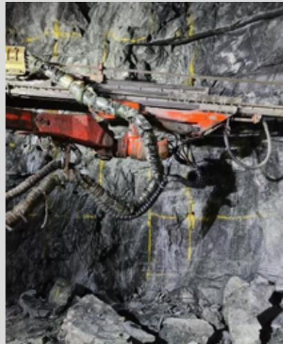
ground support was only installed on the side wall leaving the face unmeshed.
