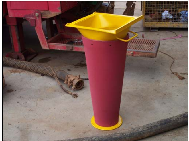
Photograph 2: New cone, which is much longer than the original cone
