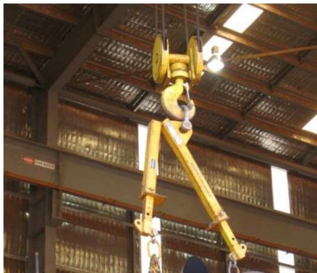
Photographs showing broken beam after lift (left) and placard indicating WLLs when being used as a spreader beam and lifting beam of various lengths.
