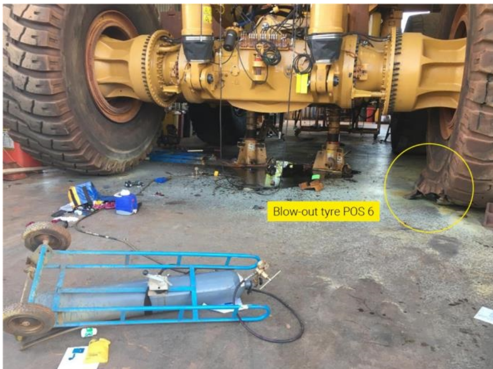
Photo of the haul truck showing the blown out tyre fitted in position 6. Tools and equipment are in their original positions.
