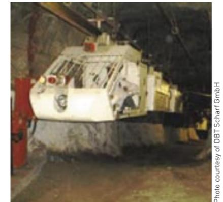
A monorail operating in a mine tunnel
