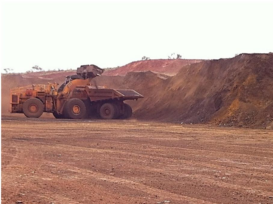
*Note: A stockpile face is “undercut” when the toe or base is advanced more than the overall face or slope. A face may also be undercut if loaders push materials at the base of the stockpile along, rather than towards, the face. Early warning signs of failure include visible cracking of the crest or top edge of the pile, and small rocks or particles rolling down the face.*
