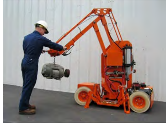
Mobile manipulators – lift and move heavy items
