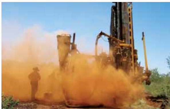
RC dry drilling
