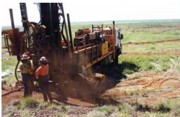
RC wet drilling (water injection)
