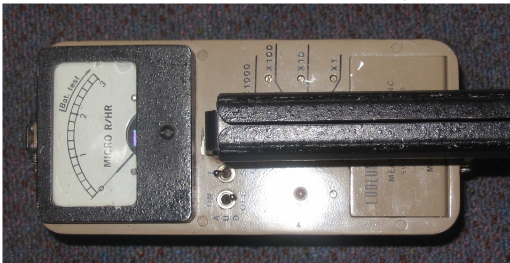
Figure B.1.: The Ludlum 12S meter reads in \mu\text{R}/\text{h}
