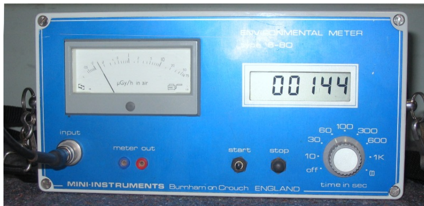
Figure B.2.: The Mini-Instruments environmental radiation survey meter reads in \mu\text{Gy/h}
