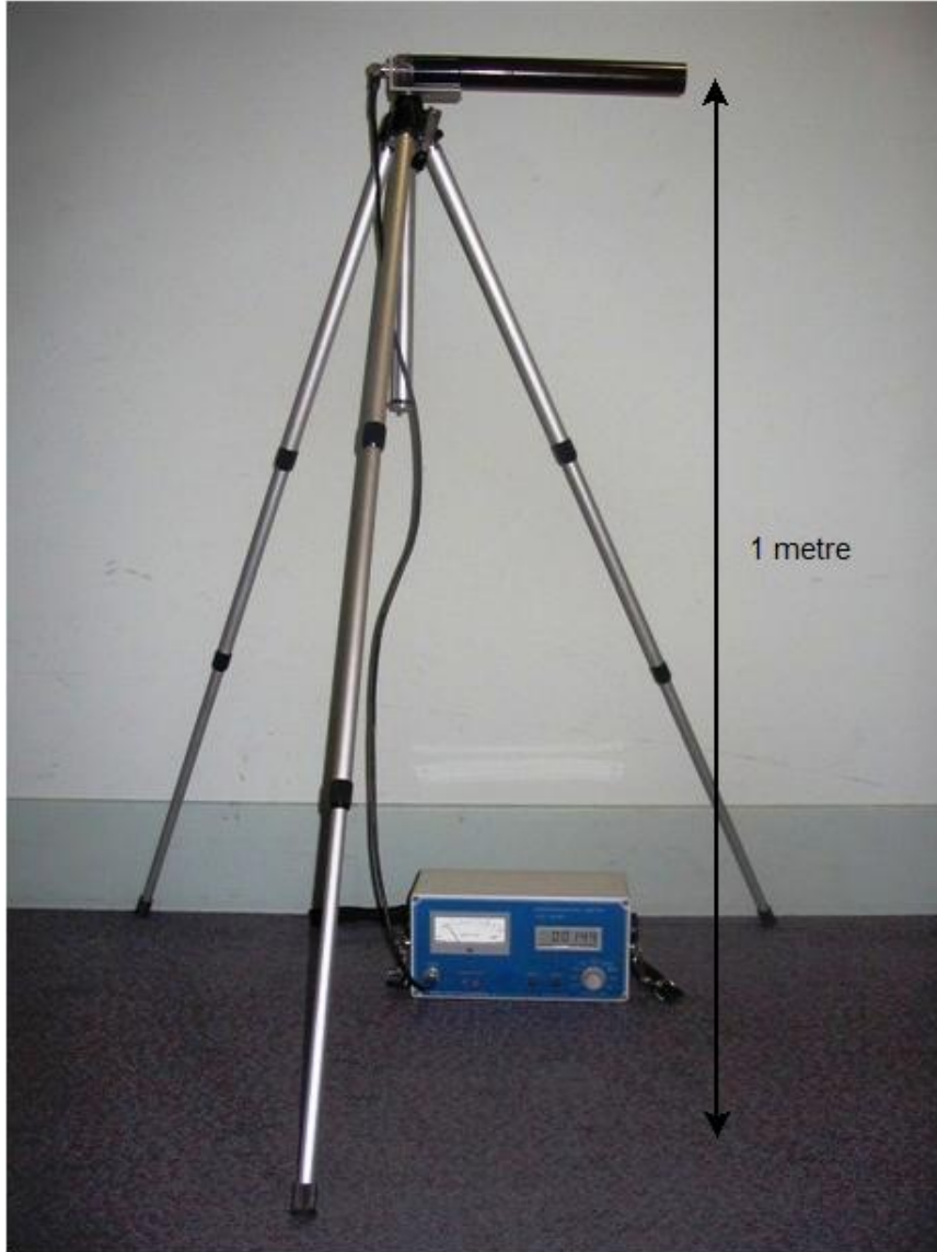
Figure 2.2.: Mini-Instruments 6-80 environmental radiation survey meter
