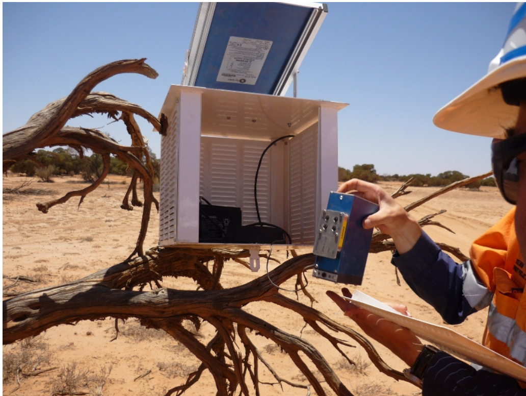
Solar/battery powered radon sampler
