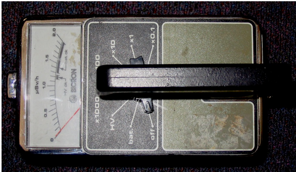
Figure B.3.: The Bicron ‘micro rem’ meter reads in \mu\text{Sv/h}
