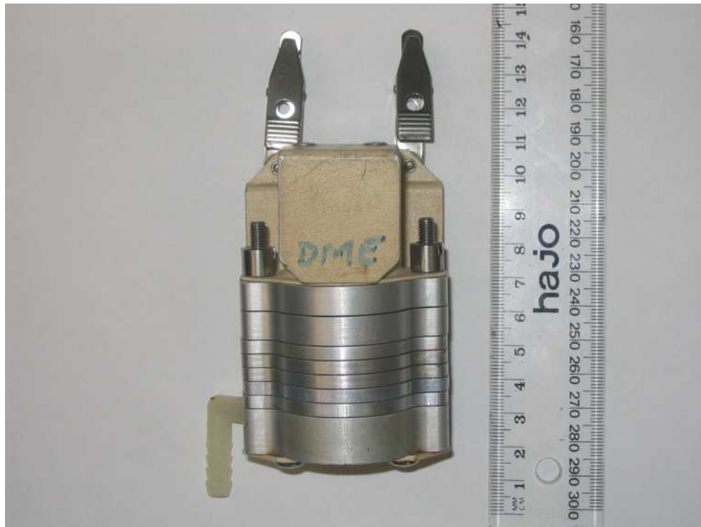
Figure 2.2.: The assembled Marple cascade impactor
